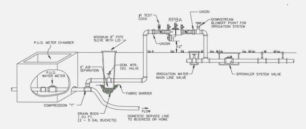
All connections to the domestic service water line must be at least 3 feet away from the meter chamber. Most domestic water lines are located 3 to 4 feet below ground. You must contact the correct water purveyor to arrange for the water to be shut off inside the water meter chamber. Entering the water chamber or shutting the water service off within the meter chamber is <u>prohibited</u>.
